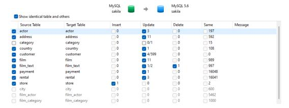
When you selected a table/collection in the list, the bottom pane shows data in the source and target. Values that differ between the source and target are highlighted. To view multiple lines data, right-click the grid and select **Show Assistant Viewer**. Uncheck the records that you do not want to apply to the target.
