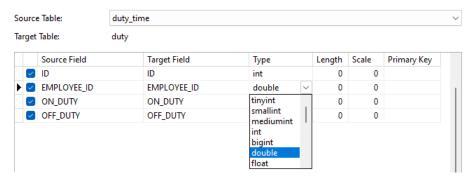
If you are importing data into existing tables/collections, you might need to map the source field names manually to the target, or right-click and select **Smart Match All**, **Direct Match All** and **Unmatch All** from the pop-up menu for quick mapping.
