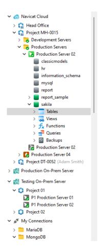
Table elements, such as fields, indexes and foreign keys, are display under each table. Click the arrow to the left of the table name to expand the list. If the elements are hidden, enable the **Show objects under table in navigation pane** option in the Options window.
