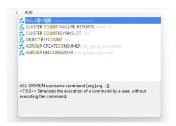
When the suggestion list appears, press TAB to insert the first item. You can also select the needed item using UPPER ARROW or DOWN ARROW and then press TAB or ENTER.
