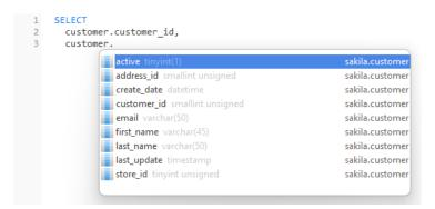
In addition, code completion can be invoked by typing a character or pressing ESC on your keyboard for SQL keywords/database objects.
